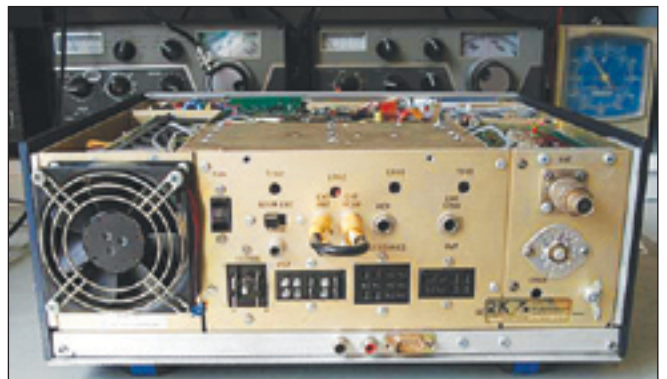
Figure 8 — TR-7 with rear extension installed.
